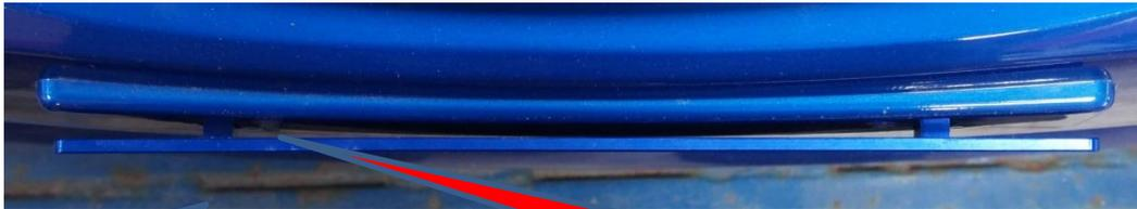
1. Align Tag Delete. The raised threaded bosses go inside the existing bumper holes.
