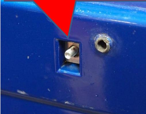
7. Screw one side of the tag bracket in. Do not tighten. Repeat for both sides.
